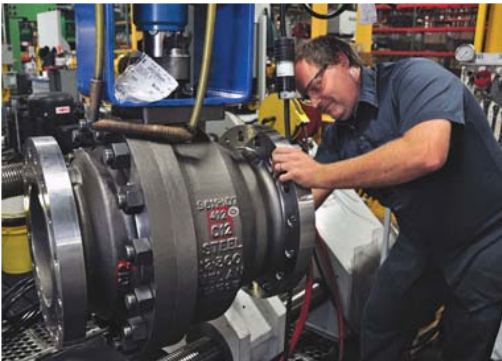
Velan's David Jones is hydrotesting a motor-operated coker ball valve. First, all electrical connections to the motor must be verified, and then the shell and back seating of the stem are tested. Finally, gasket pressure tightness tests are performed.
