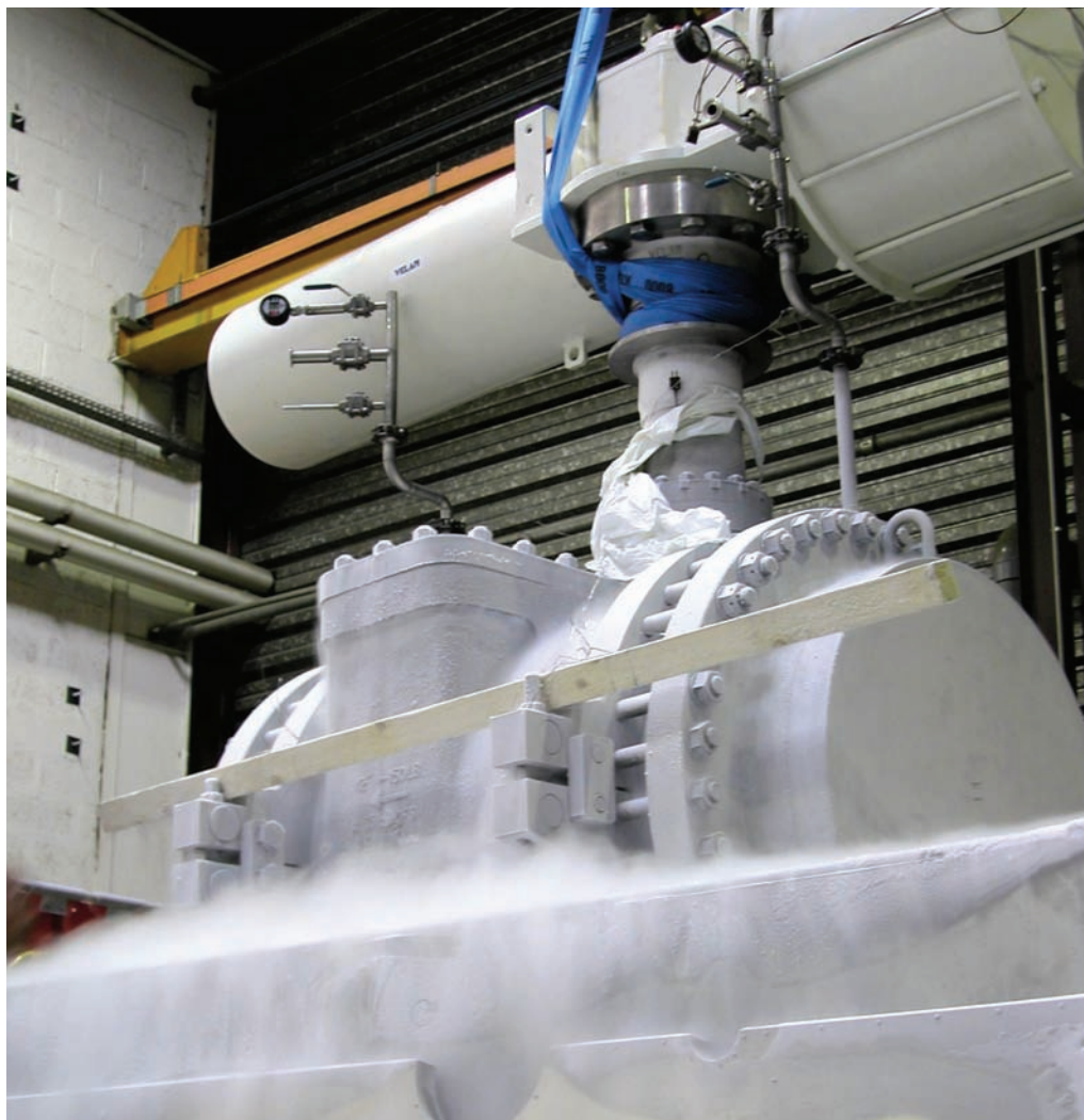
Velan cryogenic valve testing in Velan's manufacturing plant in Lyon, France.
