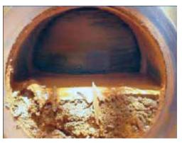
This is what the inside of a valve in an HPAL application (the type of process used on laterite ore) can look like after 24 months in service.
