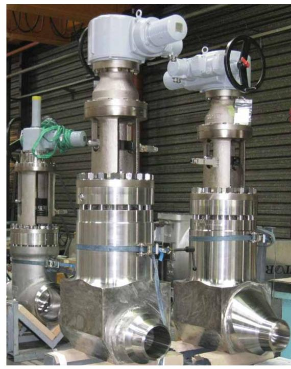
Large-size bellows seal valves ready to be shipped to the Taishan EPR<sup>™</sup> site.
