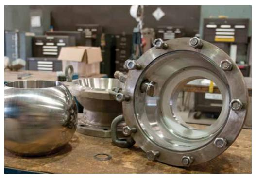
Pre-assembly of a Velan ball valve on-site.
