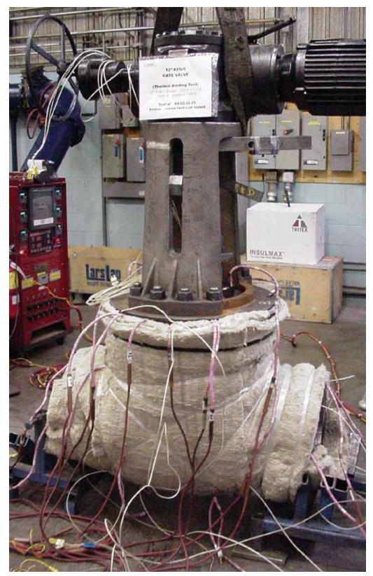
Conducting a thermal binding test on a 12" class 2500 Ultraflex wedge gate valve.
