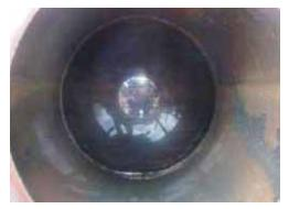
This is what the inside of a valve can look like after it has been cleaned with high-pressure water before re-installation in an HPAL application.
