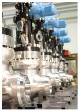
Large forged gate valves lined up for Taishan.
