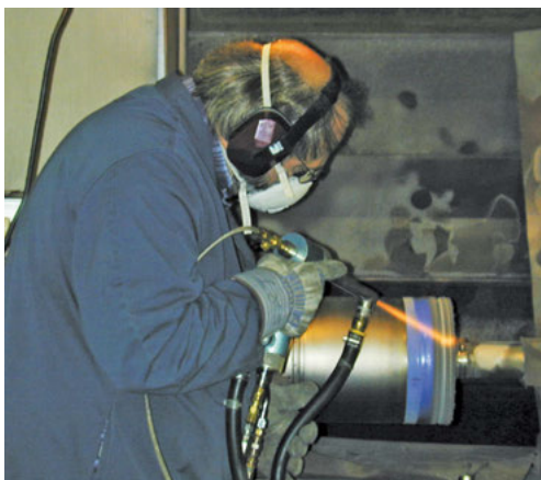
Dave Lee, Deloro Stellite's HVOF Business Manager, spraying piston ring grooves with JK®591H (NiCrMo alloy) via Jet Kote® HVOF.
