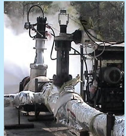
Loop isolation valve blowdown test with hot pressurized water of Velan electrically actuated NPS 8 (DN 200) class 900 regular port loop isolation valve. The water flashes to steam in a starburst pattern as it blows down to atmosphere.
