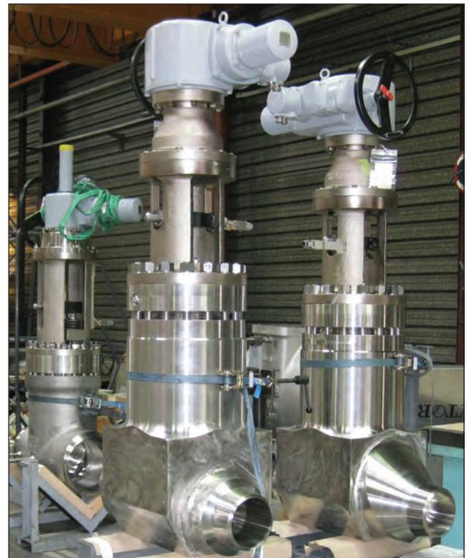
Large forged bellows seal valves for a Chinese nuclear power plant.
