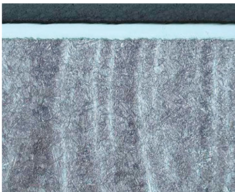
A micrograph of Hardide coating on austenitic stainless steel.
