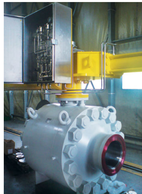
An 18" (450mm) full bore class 2500 ESD valve complete with a hydraulic SY actuator and manual PST device for offshore severe service.
