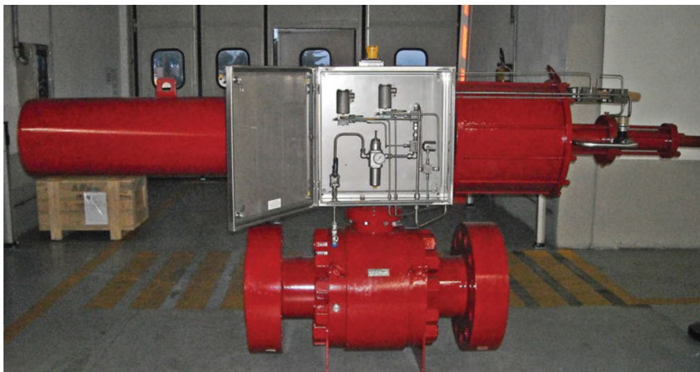
A Velan ABV HIPPS system showing the open logic control panel.
