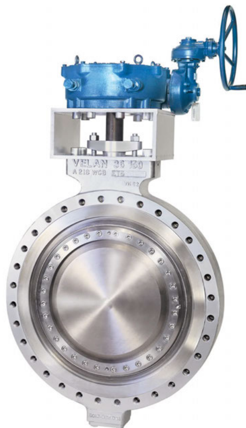
Velan's Torqseal triple-offset butterfly valve with CVD tungsten carbide-based coating on all wetted trim parts for severe service applications.
