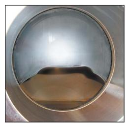
Ball with ceramic coating in half open position, after several months in service
