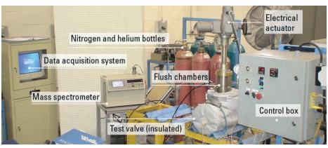
Figure 2 - Fugitive emissions testing in action.
