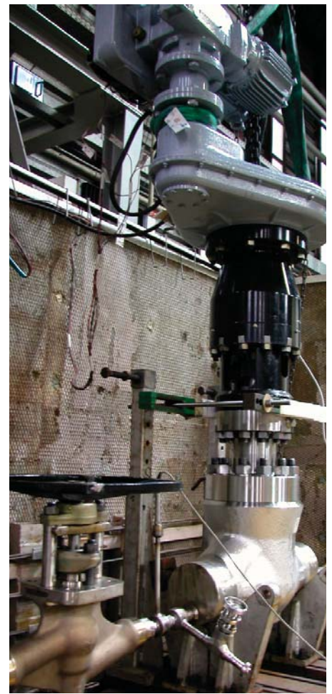
Velan supplied the first contract for nuclear bellows seal valves in 1958. Today's EPR RAMA bellows globe valve is cobalt free and offers state-of-the-art fugitive emissions control and in-line reparability.
