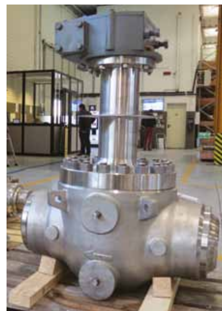
Part of a package of cryogenic ball valves from 6-24", ASME 900 class, temperatures to -196 °C, destined for an LNG project.
