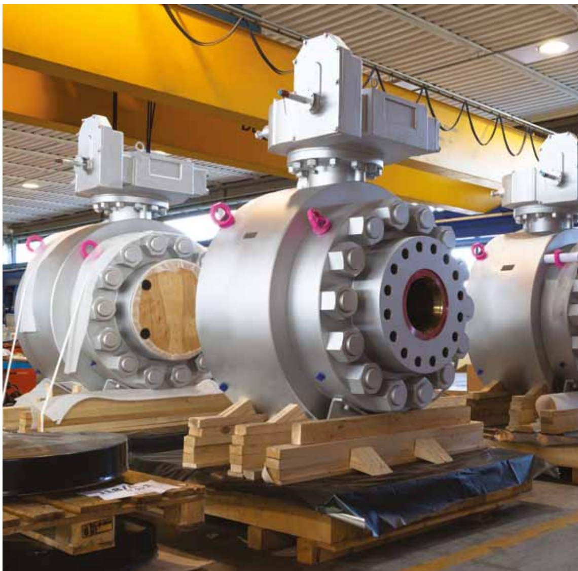
16 inch compact API 10000 ball valves for floating production storage and offloading (FPSO) topside service
