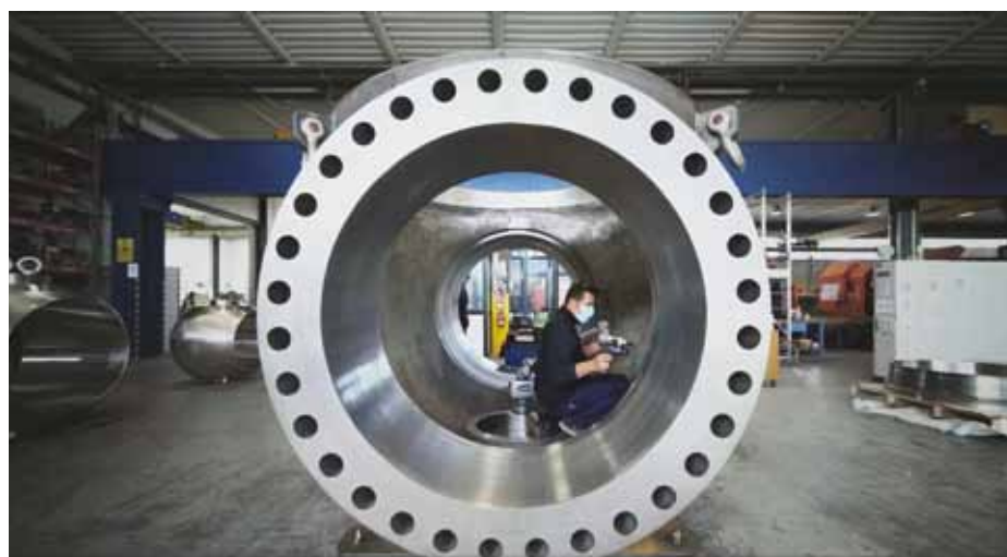
Velan ABV employees perform NDT and dimensional tests on a 52" ball valve using a ScanArm and 3D digitalization software to maximize the efficiency of the process.
