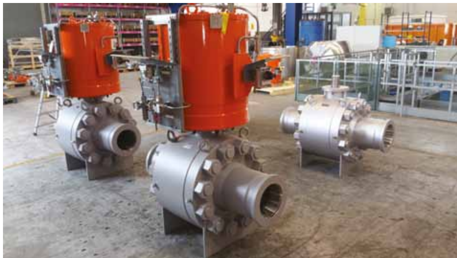
Final assembly of an API 6A side-entry ball valve
