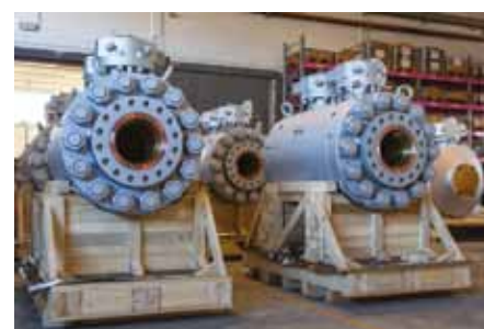
Double block and bleed ball valves API 10000 and Class 2500 for FPSO topside service
